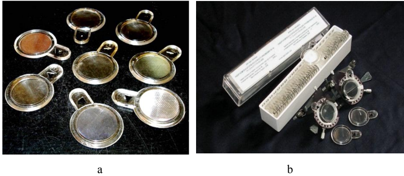
Figure 1. Microprism optical compensators and total view of diagnostic set KK-42
