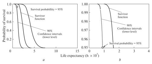
Fig. 6.7. Probability-of-survival function at 30 °C / 60%RH (a), expanded scale (b)
