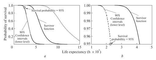
Fig. 6.6. Probability-of-survival function at 25 °C / 50%RH (a), expanded scale (b)
