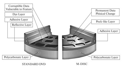
Fig. 5.4. Structure comparison of standard DVD and M-Disc [98]
