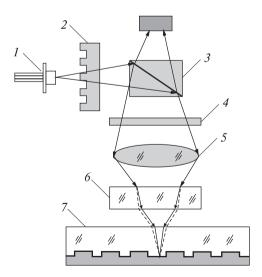
Fig. 5.27. Modified optical scheme of readout system
