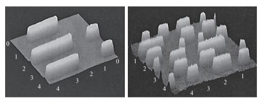
*Fig. 5.34.* Information recording area with different recording density: CD format (track pitch of  $1.6\mu$ m) (*a*); DVD format (track pitch of  $0.74\mu$ m) (*b*)
