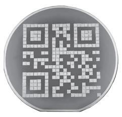
*Fig. 5.12.* Design of the HDP disk. Each pixel in the large QR codes consists of a micro-QR code [114]
