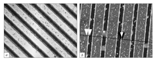
*Fig. 4.9.* Guide tracks on the optical disc carrier with  $Te_{14}Sb_{10}Se_{61}Ge_{15}$  recording medium (track pitch is 1.6 µm). The images are obtained using: a — optical microscope; b —scanning tunnel microscope [183]
