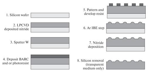
Fig. 5.10. Design of the HDP disk. Each pixel in the large QR codes consists of a micro-QR code [105]
