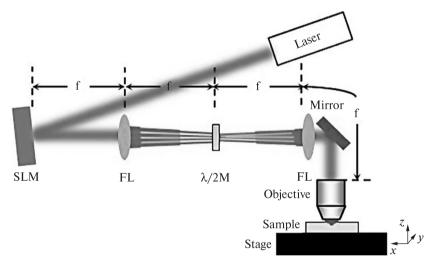
*Fig. 5.17.* 5D optical storage writing setup: femtosecond laser, spatial light modulator (SLM), Fourier lens (FL), half-wave plate matrix (L/2 M), dichroic mirror, 1.2 NA water immersion objective, silica glass sample, translation stage [163]
