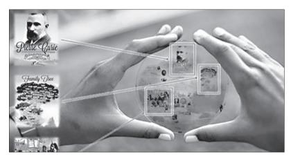
Fig. 5.21. A hard disk from sapphire of the Fahrenheit 2451 project
