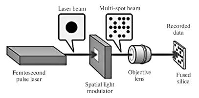
*Fig. 5.15.* The concept of storing data optically in the bulk of non-photosensitive transparent materials [162]
