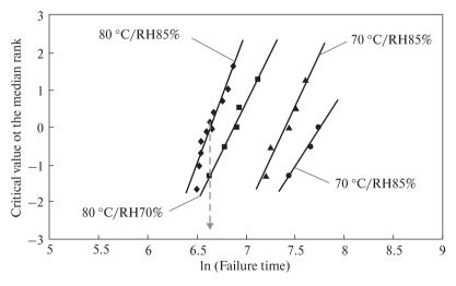
*Fig. 6.3.* Relation between the limit value of F(t) for the median rank of lifetime data and the natural logarithm of the lifetime data [94]
