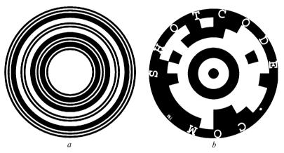
Fig. 2.2. Circular barcode structure: a - Circular 1D barcode, b - ShotCode
